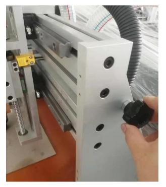
12.Position the cardboard with the positioning block and lock the locking screws.
