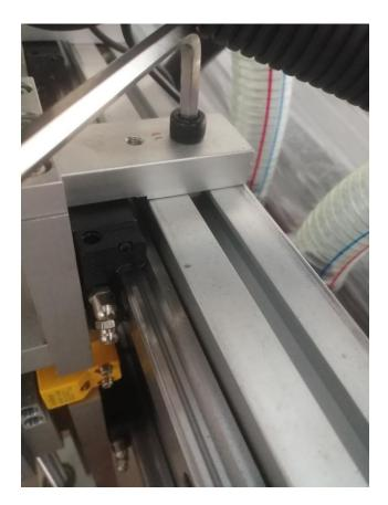
11.Turn "the adjustment handle" and adjust the cardboard position so that the drill bit is well positioned for drilling the cardboard.
